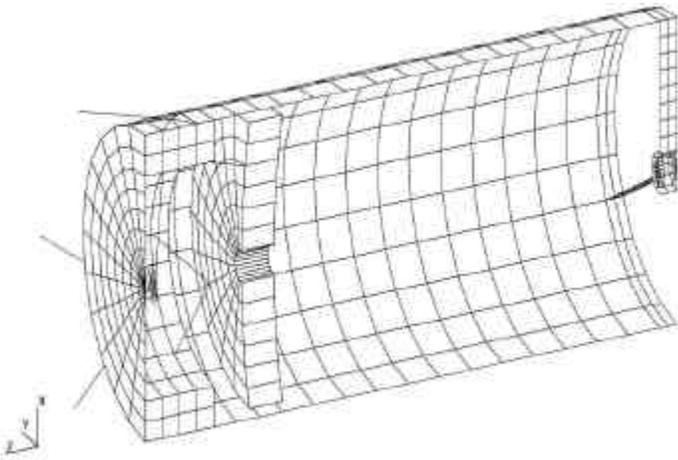
Figure 1: Cut-away View of NASTRAN Model
