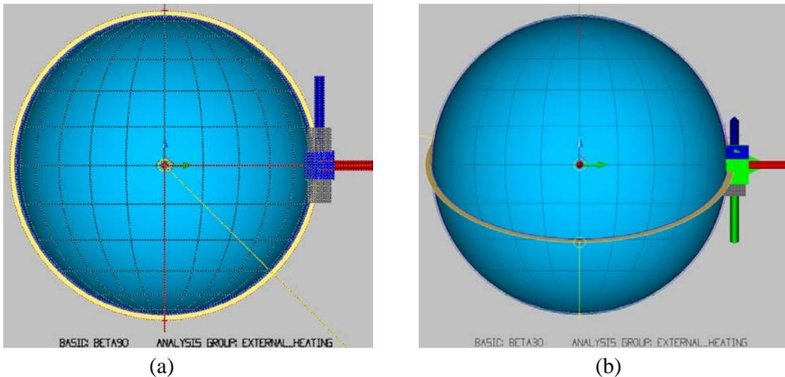
**Figure 2-5** (a) CubeSat Orbit for beta angle = 90 deg. (b) beta angle = 30 deg.
