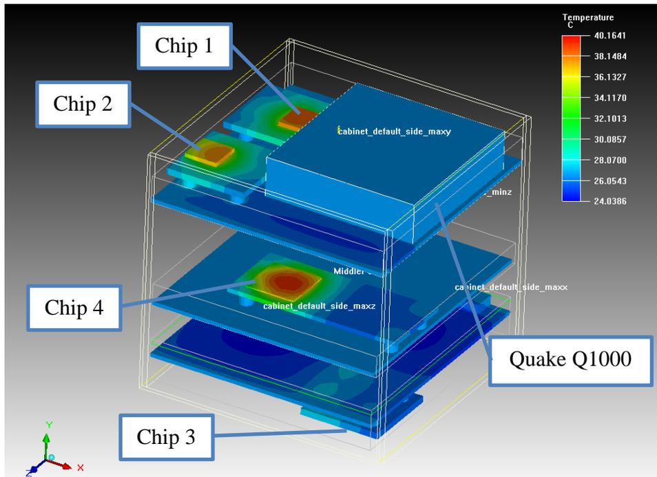
Figure 5-4 CubeSat Temperature Profile – Hot Case Analysis
