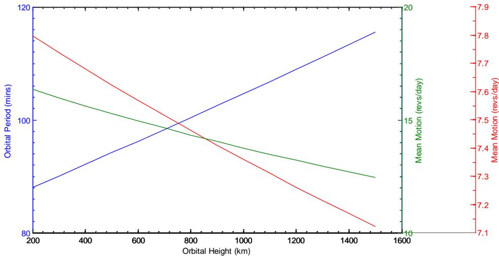
**Figure 2-3** Orbital Parameters for Low Earth Orbit
