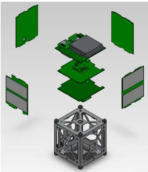
**Figure 3-1** Example of a CubeSat Model – Exploded View
