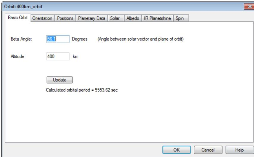
2. The orientation and positions of the satellite can be changed under the Orientation and Positions tabs. For CubeSat operating in LEO, the Earth parameters were used under Planetary Data tab.
