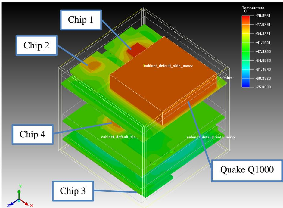
**Figure 5-5** CubeSat Temperature Profile – Cold Case Analysis
