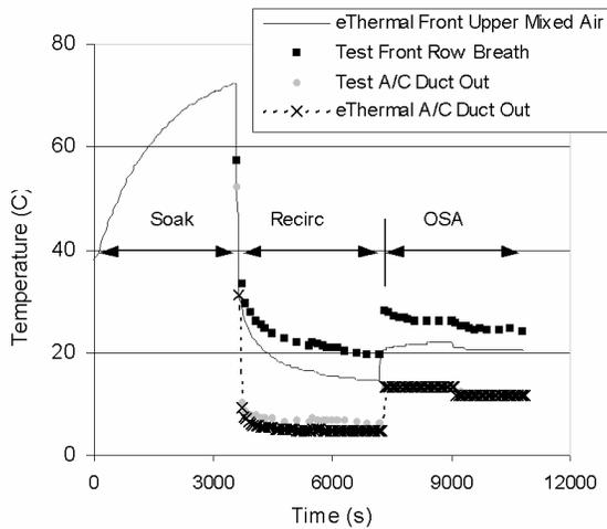
Figure 20 Soak and cool down: Temperatures
