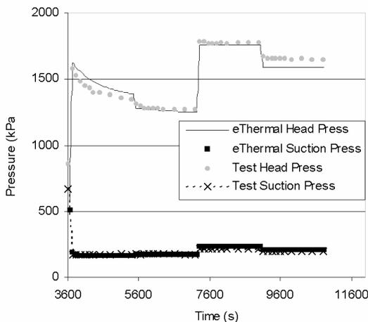
Figure 21 Soak and cool down: head pressures and suction pressures
