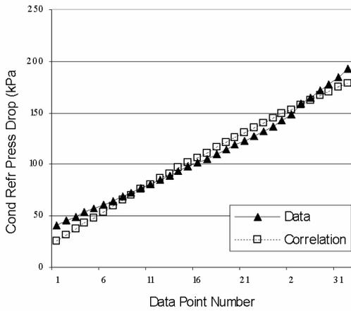
Figure 5 Condenser refrigerant pressure drop correlation
