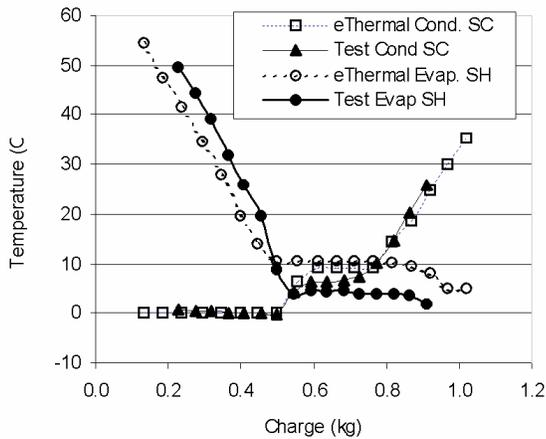
Figure 18 Variation of evaporator outlet superheat and condenser outlet sub-cooling with system charge
