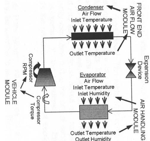
Figure 2 Boundary Conditions for A/C system
