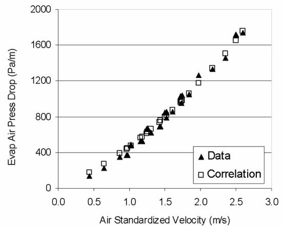
Figure 9 Evaporator air side pressure drop correlation
