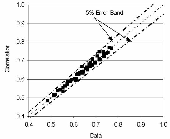
Figure 11 Compressor volumetric efficiency correlation
