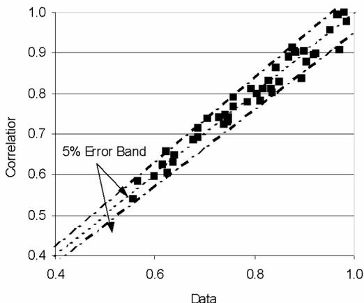
Figure 10 Compressor isentropic efficiency correlation
