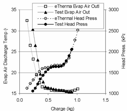
Figure 17 Variation of head pressure and evaporator air discharge temperature with system charge
