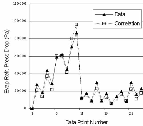
Figure 8 Evaporator refrigerant pressure drop correlation
