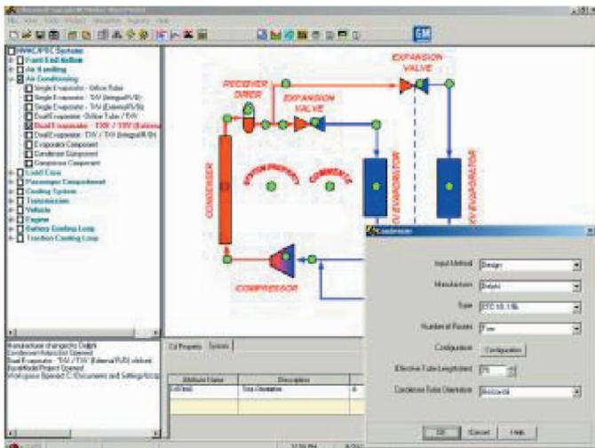
Figure 1 e-Thermal Graphical User Interface
