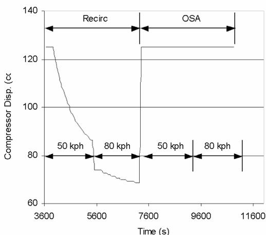
Figure 22 Soak and cool down: Compressor displacement
