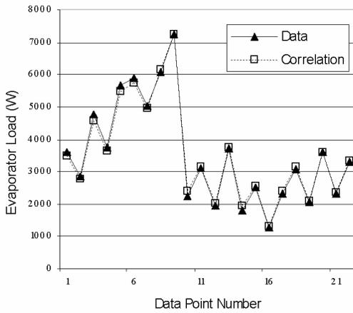
Figure 7 Evaporator heat transfer correlation
