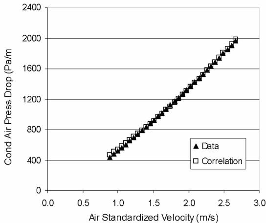
Figure 6 Condenser air pressure drop correlation
