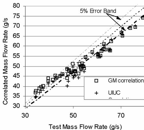
Figure 13 Orifice tube mass flow rate correlation
