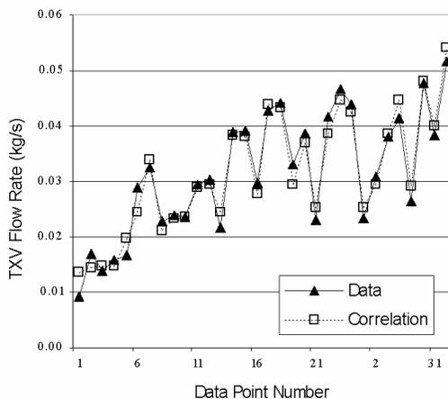
Figure 15 TXV mass flow rate correlation
