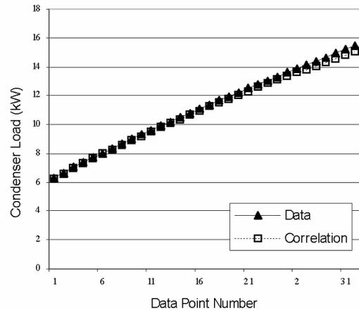
Figure 4 Condenser Heat Transfer Correlation
