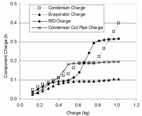
Figure 19 Refrigerant distribution in various components as a function of system charge
