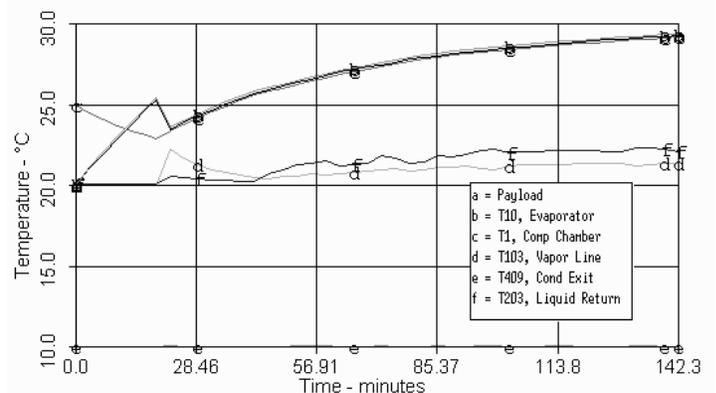
conductance shows that 10 watts is insufficient in offsetting the wick back conduction and subcooling associated with 25 inches of adverse tilt.
