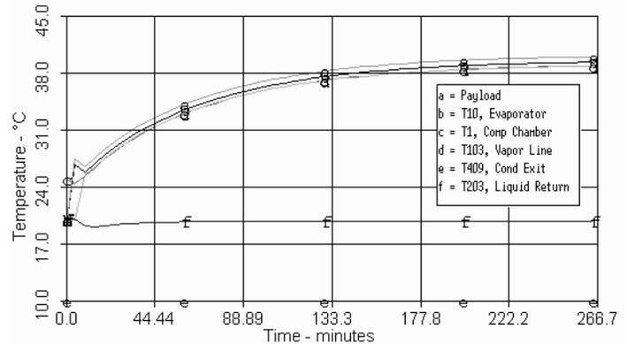
**Figure 9: Startup with 50 Watt Load, Heat Flow Summary**
