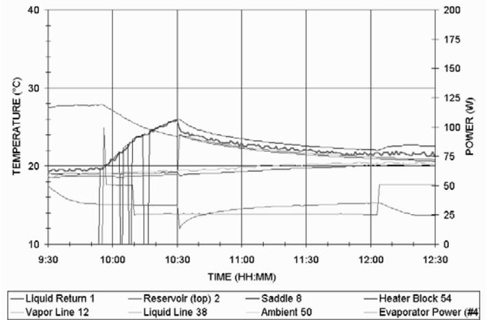
Figure 12: Reverse Flow at LHP Startup (Test Data)
